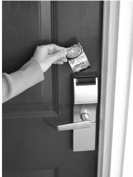
■ FIGURE 16.2 First generation access control reader.
