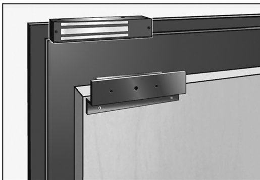
■ FIGURE 11.3 Inswinging door configuration. Image courtesy of Security Door Controls.
